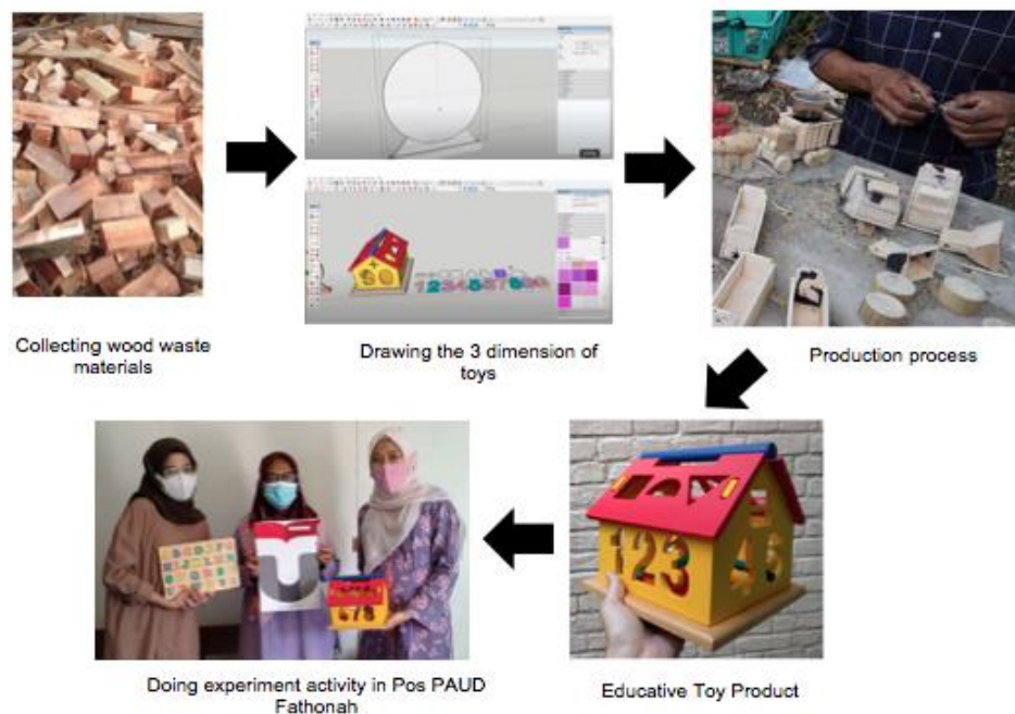
Figure 2. Producing an Instrument of Educational Toys from Wood Waste Materials [Source. Personal Document, 2021]
